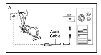
B. Plug one end of the audio cable into the jack beneath the console of the elliptical crosstrainer. Plug the other end of the cable into a 3.5mm Yadapter (available at electronics stores). Plug the Yadapter into the PHONES jack on your computer. Plug your headphones or speakers into the other side of the Y-adapter.
